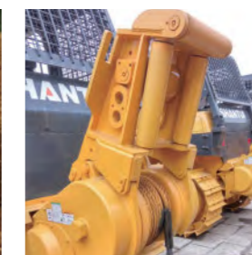
*Hydrostatic winch can be used for self rescue, equipment recovery, logging, or other maneuvers. The SHANTUI hydrostatic winch features excellent line pull at any speed and infinitely variable drum speed.
