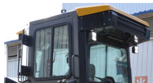
*Four forward and two rear high-intensity halogen work lights are positioned high for nearly 360 deg superior illumination to extend your workday beyond daylight.
