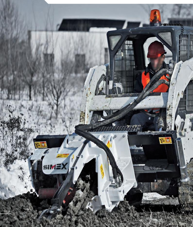
Designed for fixed-section trenching on soft soil.
