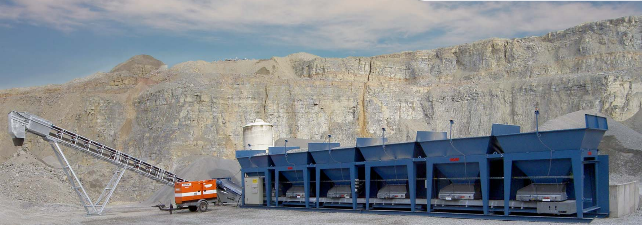
Photo : Euromix 406/6 with a 16,5m fixed loading conveyor
